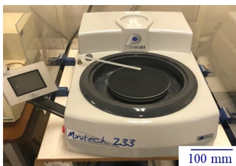
Fig. 2.8 Polishing machine (MI-233-A/J15, Meiwafoosis Co. Ltd.)
