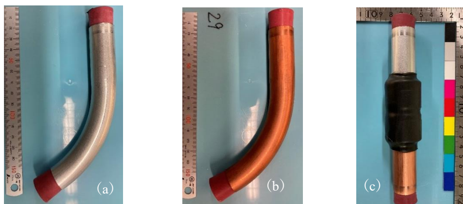
Figure 5-1 Appearance for test samples (a) bent Aluminum pipe (Al), (b) bent Copper pipe (Cu), (c) connecting Aluminum and Copper pipe (Al-Cu).
