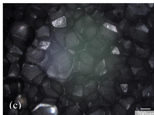
Figure 5-4 Water absorption characteristics of insulation material after immersion in a 3.5 wt.% NaCl aqueous solution for 8 hours: (a) total water absorption, (b) cross-sectional structure of PE thermal insulation, (c) cross-sectional structure of EPDM thermal insulation.
